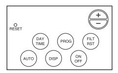
Fig. 4 - Air Purifier Control Area
